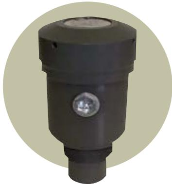
*If only a simple 4 – 20 mA output is required, a two-wire SmartSonic ultrasonic sensor may be utilized. Available in both standard and sanitary models, the two-wire model offers all of the design benefits of SmartSonic technology, but with more limited communications options. Programming is done on the sensor versus via PC software.*
